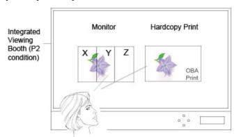
Figure 4. Soft proofing configuration in the second experiment
