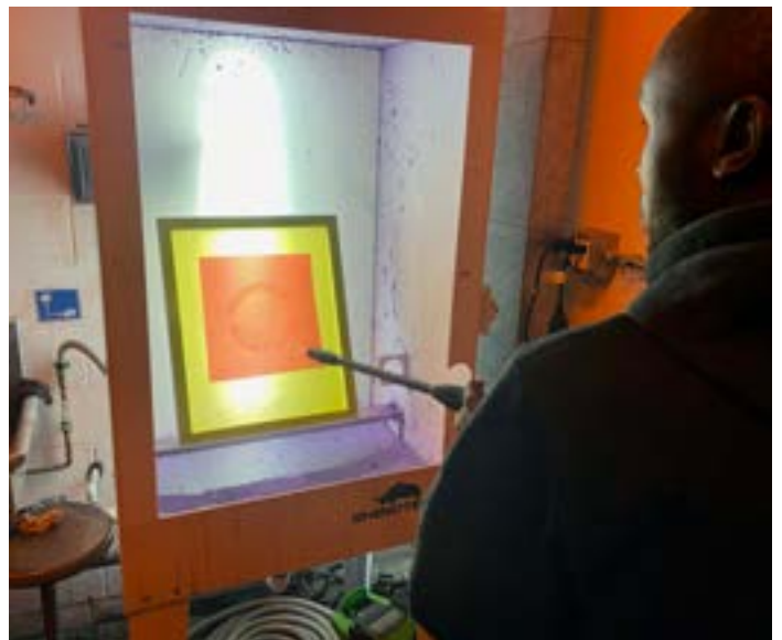
Students prepared, exposed and washed the screens
