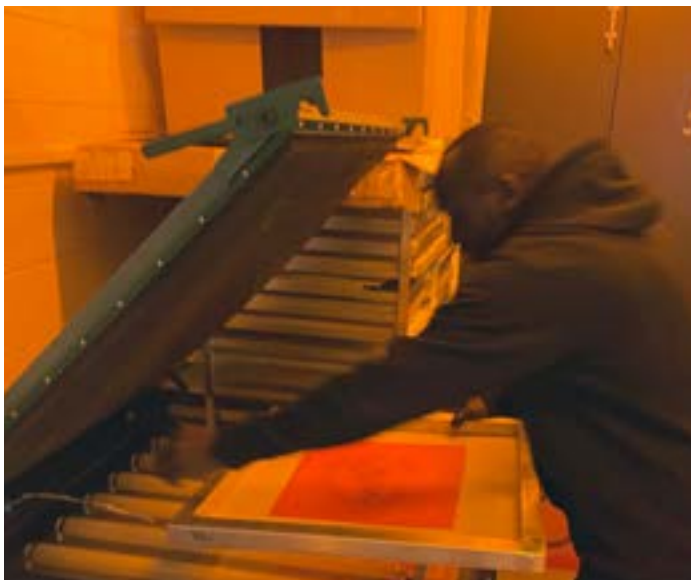
Students prepared, exposed and washed the screens
